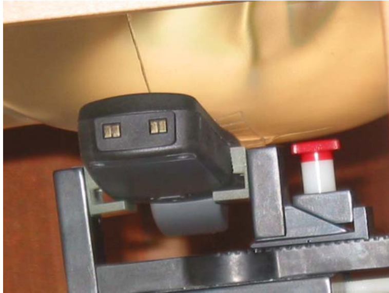
Left Head Touch Test Position
