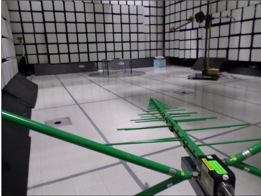
Photograph 4. Radiated Spurious Emissions, Test Setup, Below 1 GHz, Antenna View
