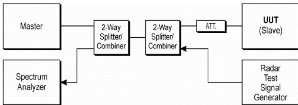
**Figure 3-1. Conducted Test Setup for DFS**
