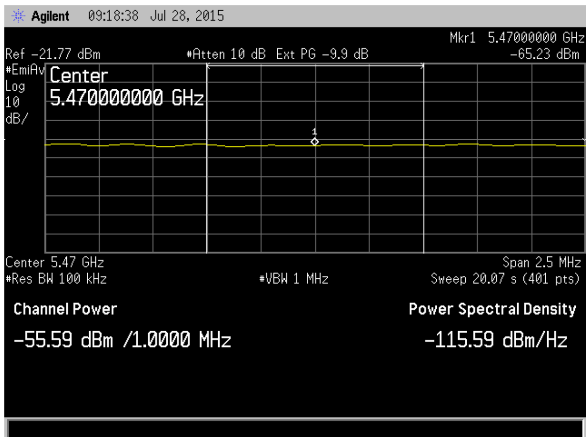
Figure 89. 5.47 GHz Band Edge Compliance 802.11n 40 MHz BW – Average
