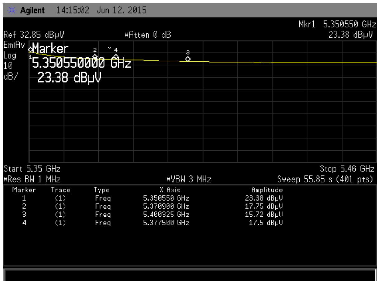
Figure 95. Restricted Band 5.35 - 5.46 GHz operating on Channel 64, 802.11a - Average
