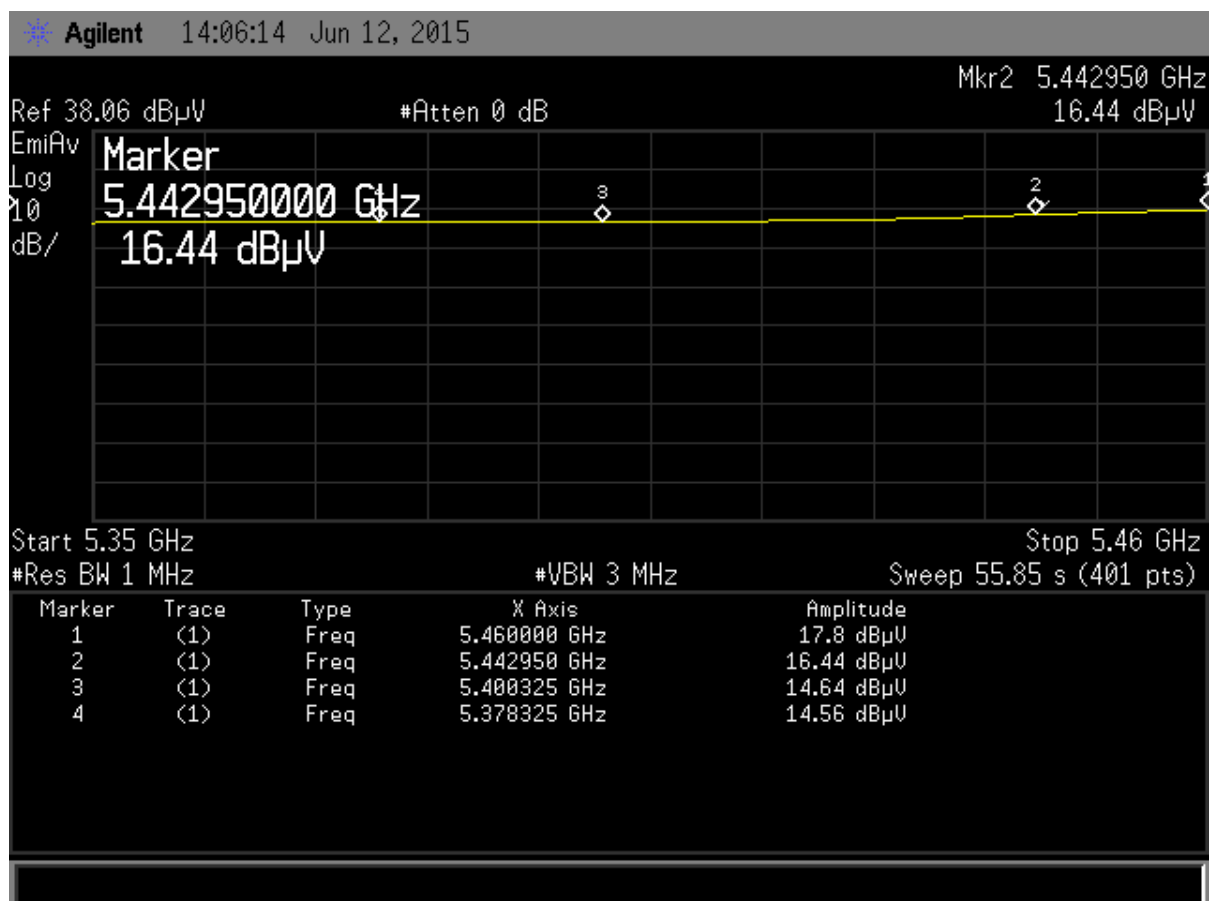
Figure 103. Restricted Band 5.35 - 5.46 GHz operating on Channel 100, 802.11n – Average
