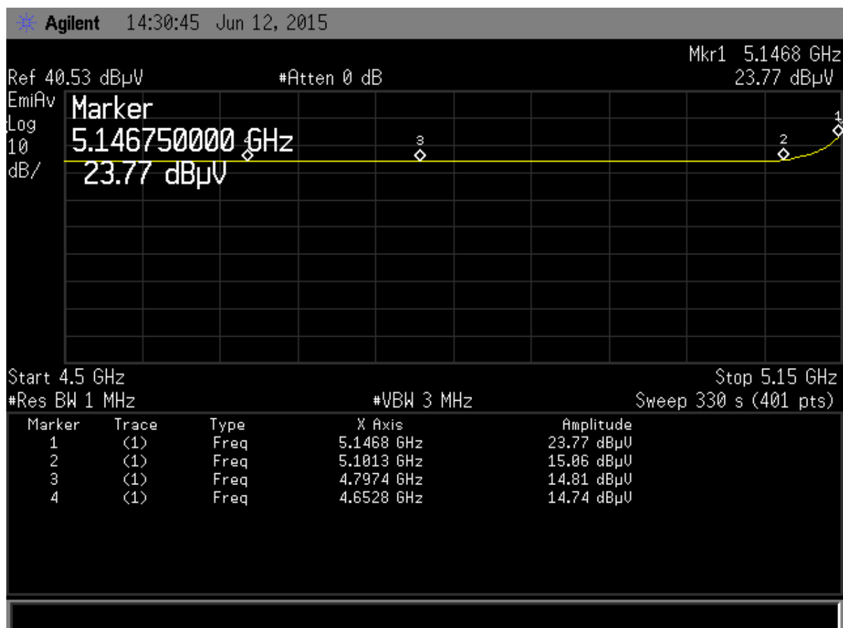
Figure 93. Restricted Band 4.5 - 5.15 GHz operating on Channel 36, 802.11a - Average
