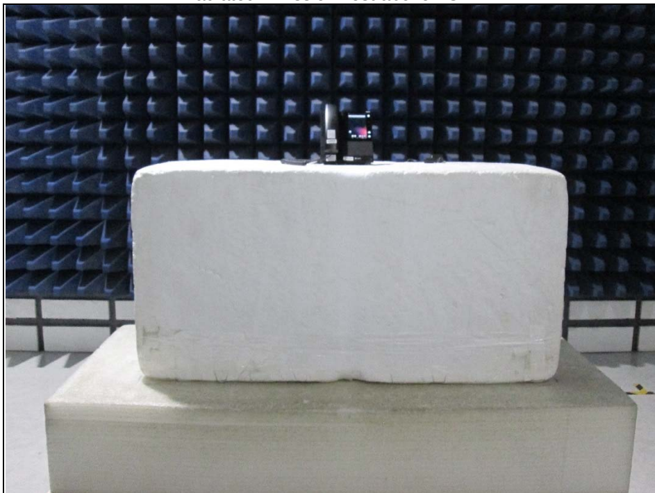
Radiated Emission Test above 1GHz
