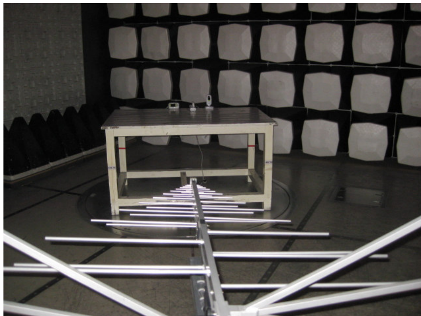
Radiated Spurious Emission Test Setup
