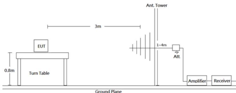
Radiated emission tests were performed in the 3 meters chamber test site, using the setup accordance with the ANSI C63.10-2013.
