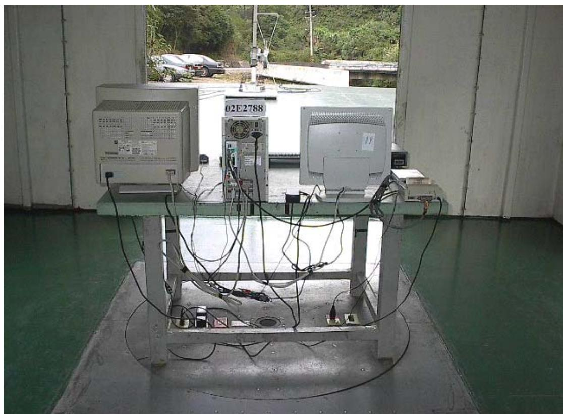
Radiated Measurement Photos Mode : LCD Monitor
