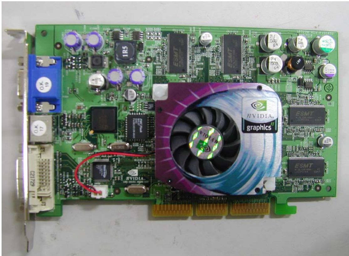
Photo # 7 Front View Rear View Mode : 8MX16X8PCS, CRT+TV+DVI
