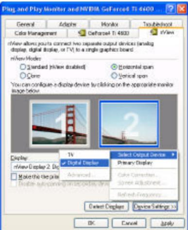
Monitor with blue frame is active. Right click on it will show the configuration menu. Or you can click **Device Settings>>** to set all the functions like "Standard mode".
