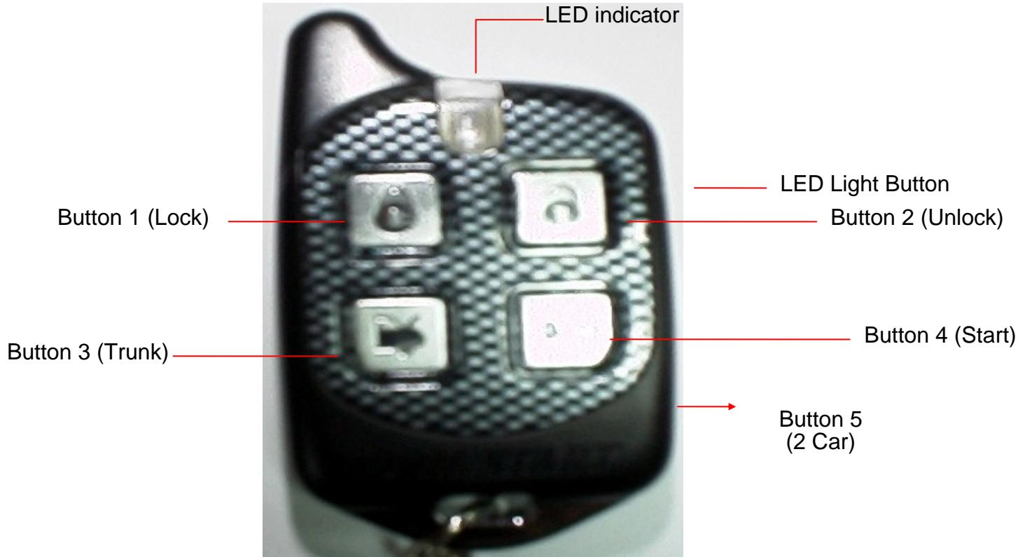
This is the transmitter of car alarm system, it use a A23 battery, the transmitter range around 100 M to 150 M.
