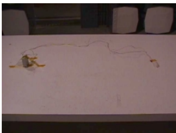
FCC MAXIMUM-RADIATED-EMISSIONS TEST CONFIGURATIONS P6EZIO 5m SEMIANECHOIC CHAMBER LEXMARK INTERNATIONAL, LEXINGTON KY.
