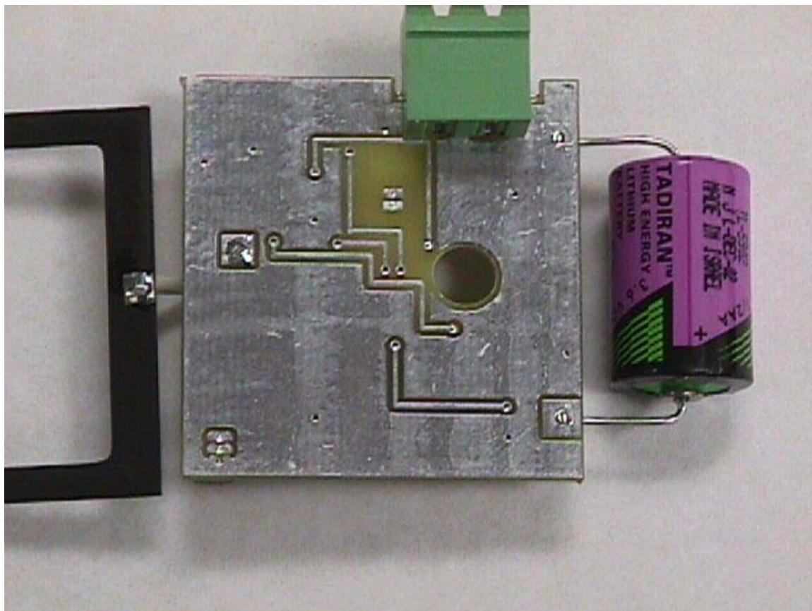
**Bottom View of the Wireless Counter/Temperature Sensor Board.**
