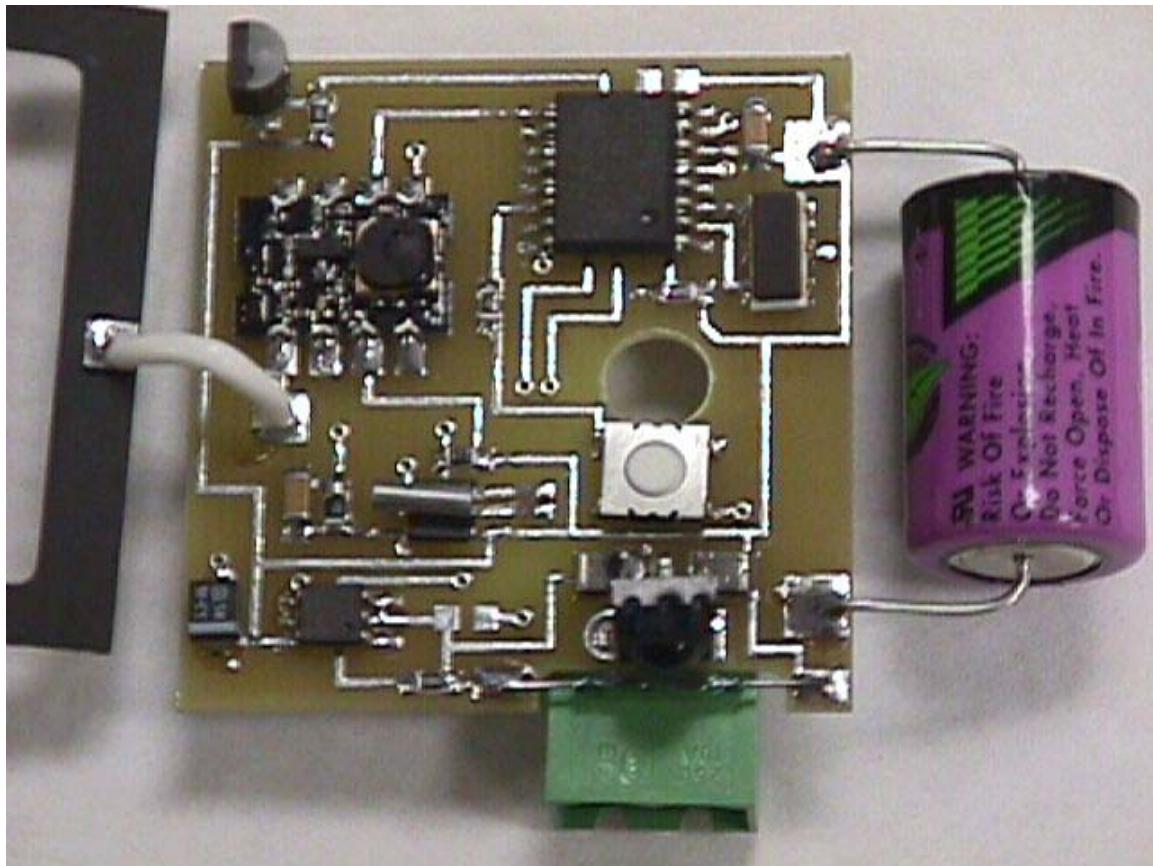
**Top View of the Wireless Counter/Temperature Sensor Board.**
