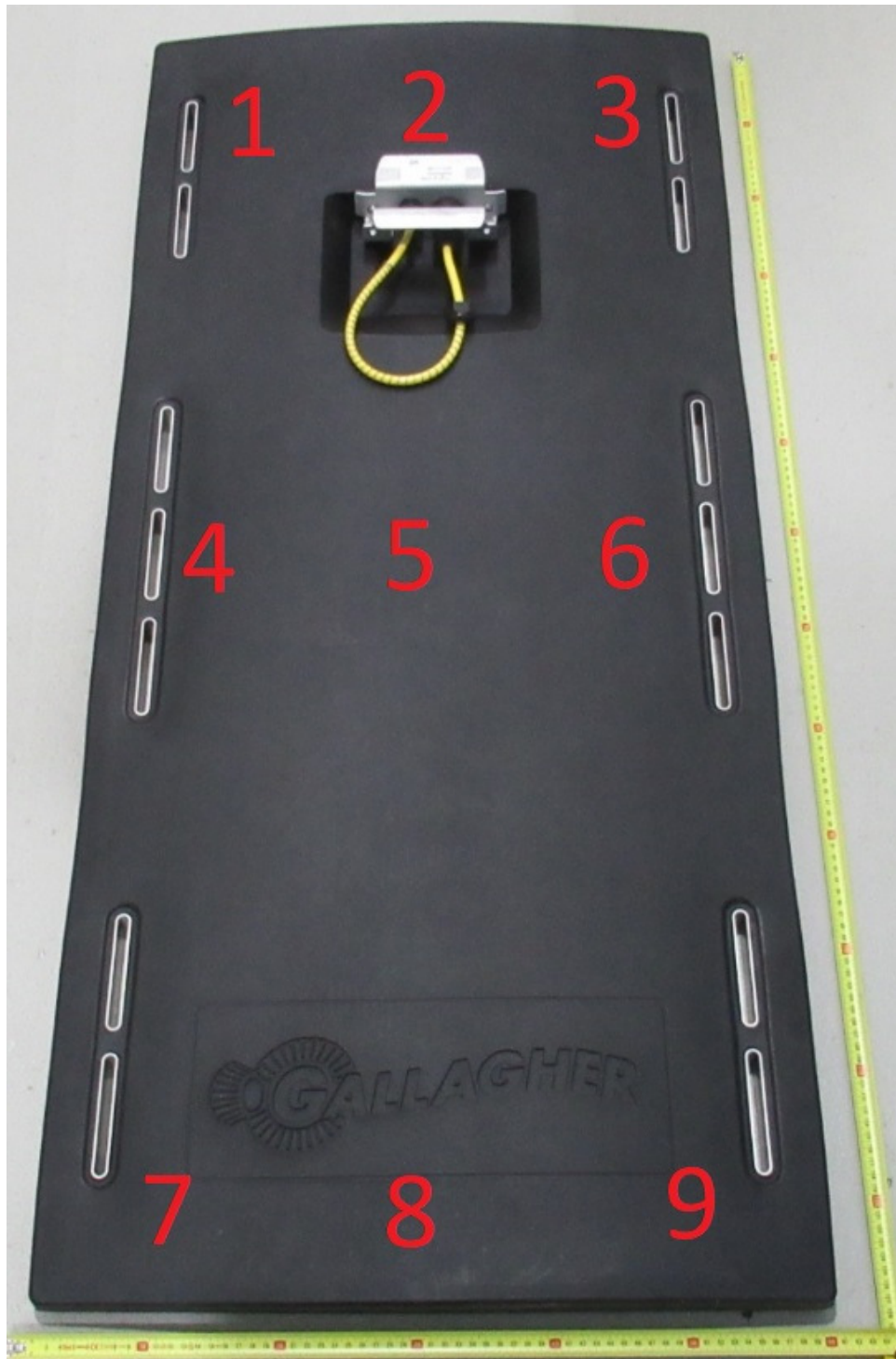
Image 1: Large Inductive Loop Antenna 1.3m x 0.6m
