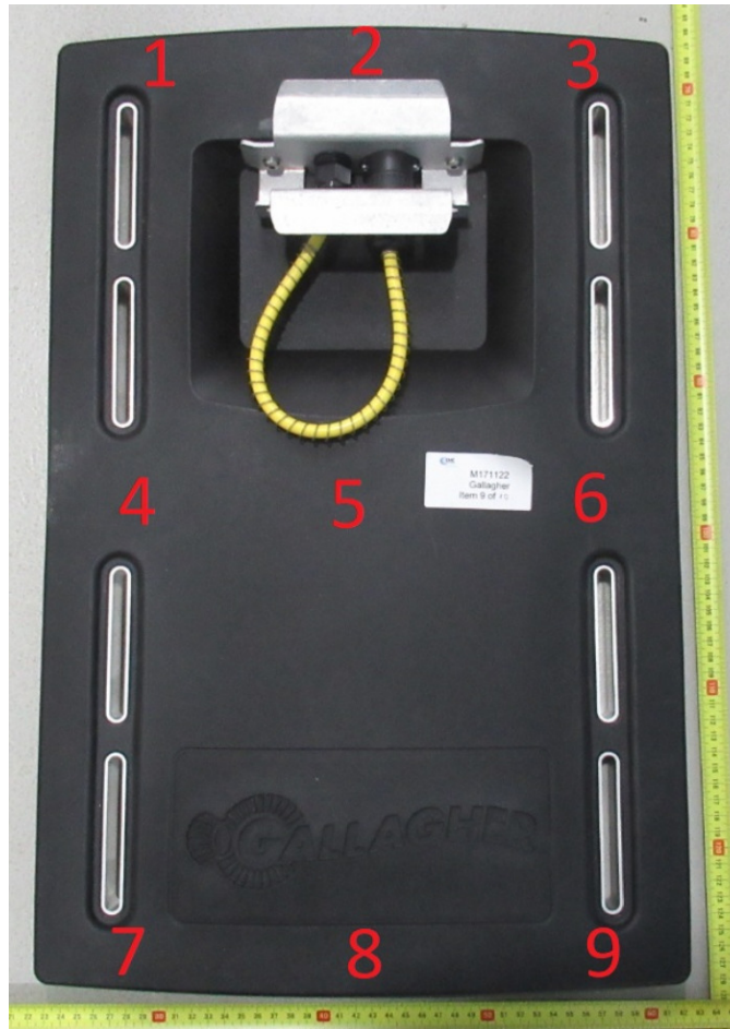
Image 2: Small Inductive Loop Antenna 0.6m x 0.4m
