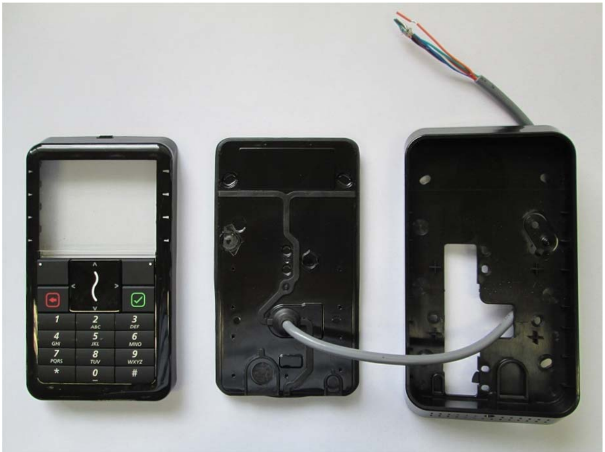
T20 Multi Tech - Front Case with Keypad, Back Cover with Connection Cable and Mounting Bracket
