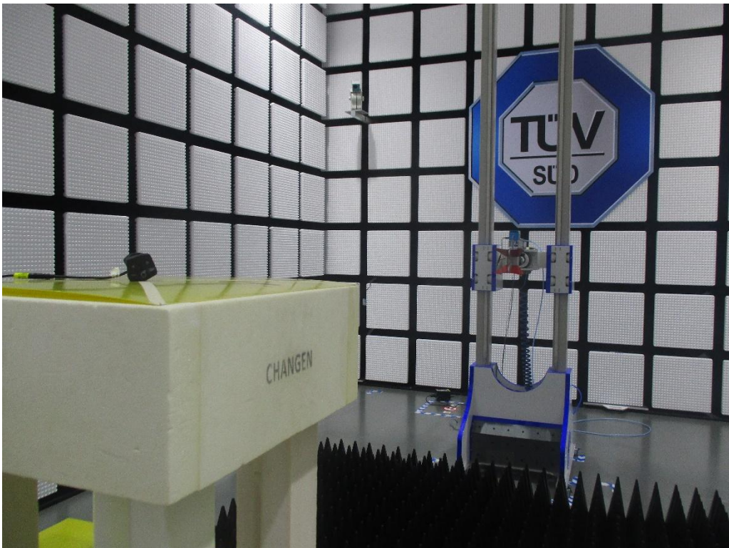
Radiated Emission Test above 1 GHz
