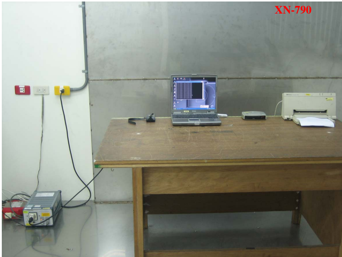
Photo 1: Conducted Emission Test Set-up photo
