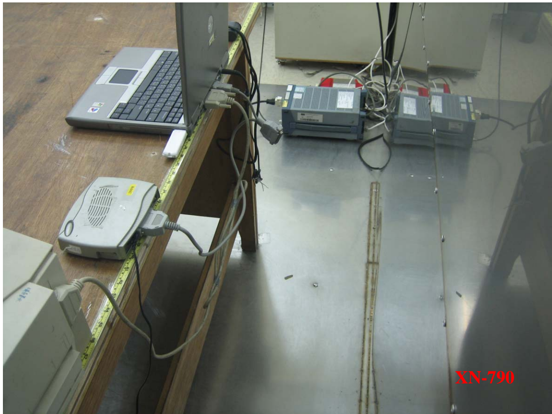
Photo 2: Conducted Emission Test Set-up photo
