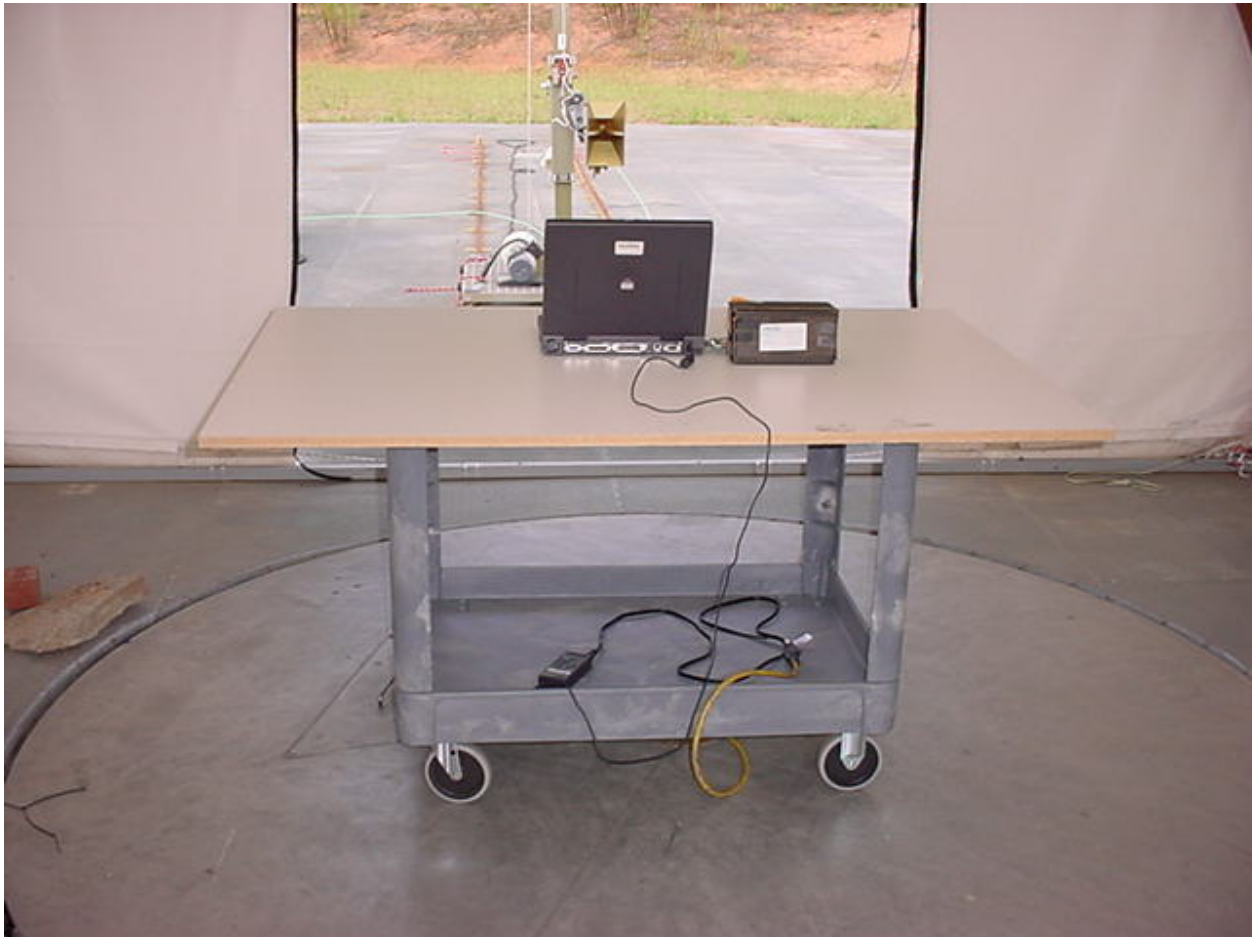
Figure 1: Radiated Emissions – Setup Rear View
