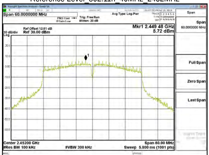
Reference Level 802.11n 40MHz 2452MHz
