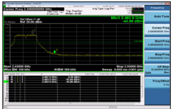
802.11g: Band Edges Test Data CH-High
