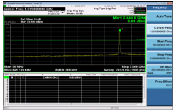
802.11n_HT20: Spurious Emission Test Data CH-Mid (MIMO)
