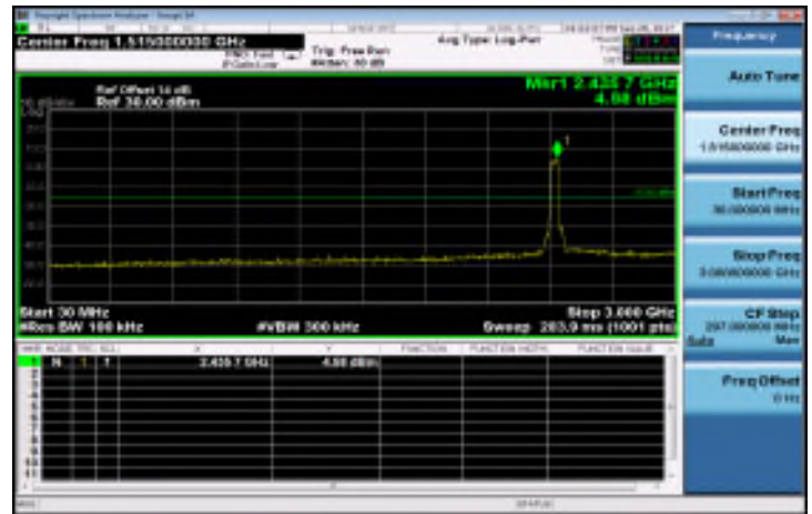
802.11n_HT40: Spurious Emission Test Data CH-Low (MIMO)
