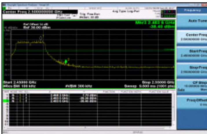
802.11n_HT20: Band Edges Test Data CH-High (MIMO)
