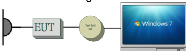
Fig. 2-2 Conducted (Antenna Port) Emission Configuration
