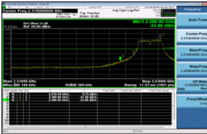
802.11n_HT20: Band Edges Test Data CH-High (MIMO)
