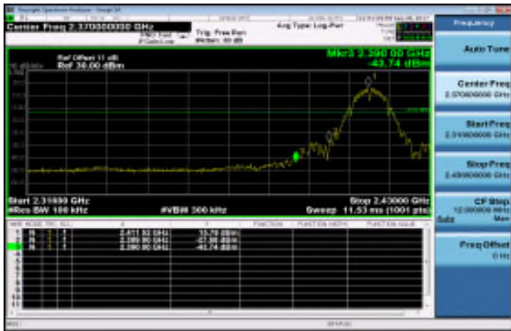
802.11b: Band Edges Test Data CH-High
