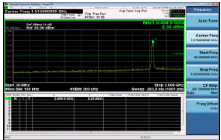
802.11n_HT40: Spurious Emission Test Data CH-High (MIMO)
