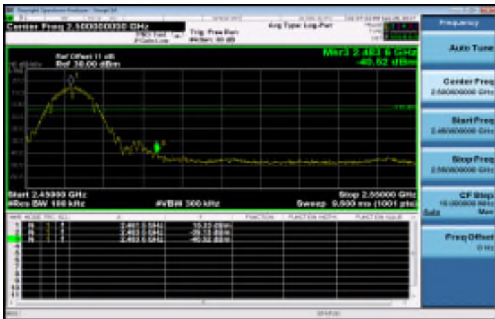
802.11b: Band Edges Test Data CH-High
