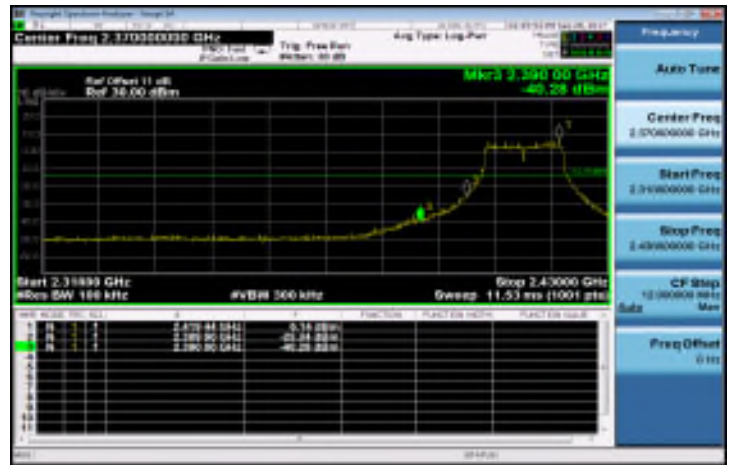
802.11g: Band Edges Test Data CH-High
