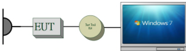
Fig. 2-2 Conducted (Antenna Port) Emission Configuration
