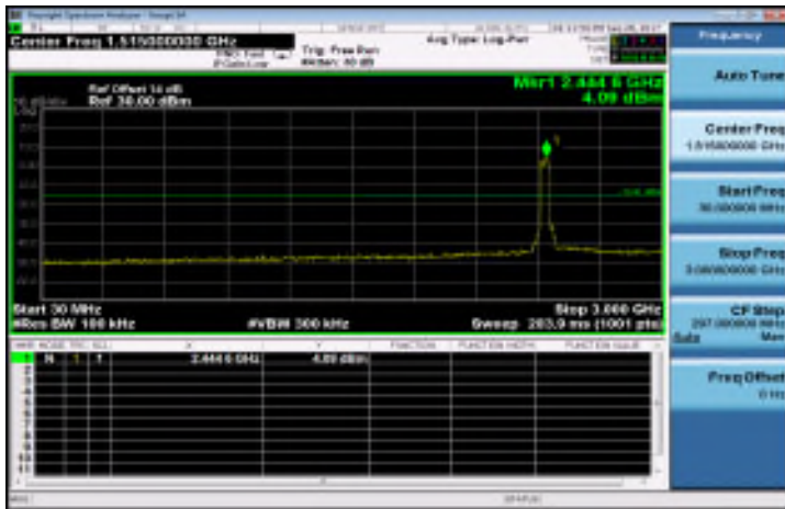
802.11n_HT40: Spurious Emission Test Data CH-Mid (MIMO)
