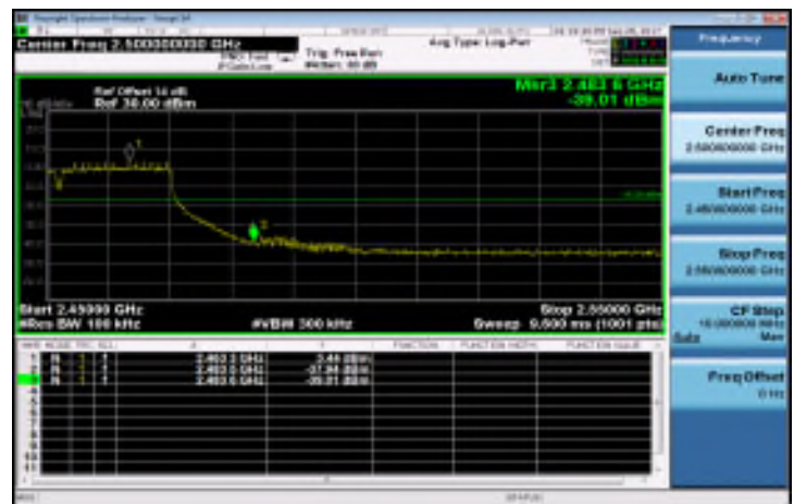
802.11n_HT40: Band Edges Test Data CH-High (MIMO)
