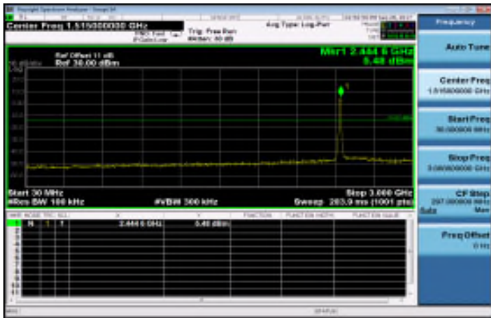
802.11g: Spurious Emission Test Data CH-Mid
