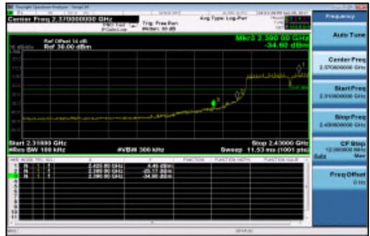
802.11n_HT40: Band Edges Test Data CH-High (MIMO)
