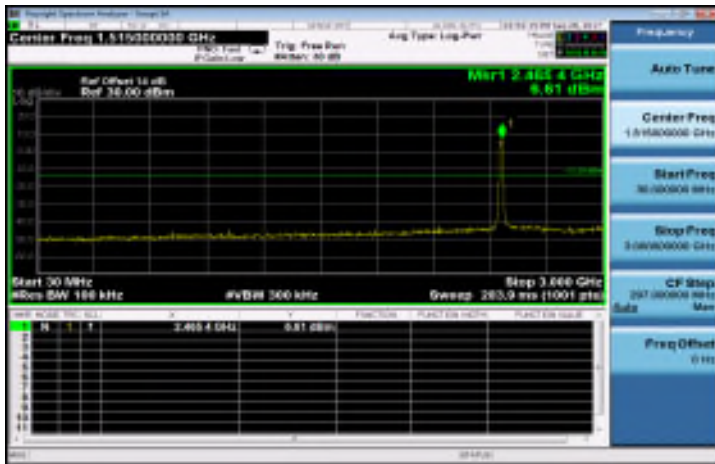
802.11n_HT20: Spurious Emission Test Data CH-High (MIMO)
