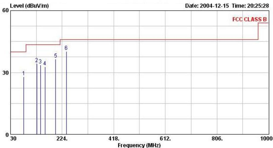
The test was performed on EUT under 802.11g continuously transmitting mode channel 1, 6, 11 were verified. The worst case occurred at 802.11g Tx channel 1.
