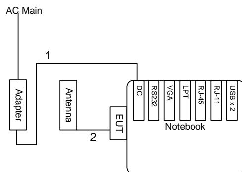
1. DC power line, 1.5m, No-shielding
