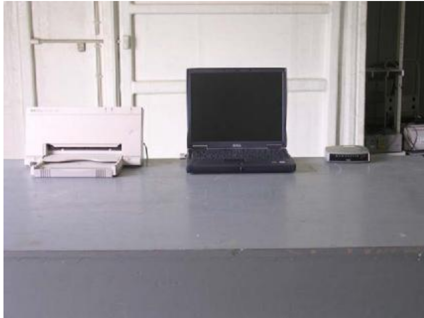
Photo 1: Radiated Emission Test Set-up
