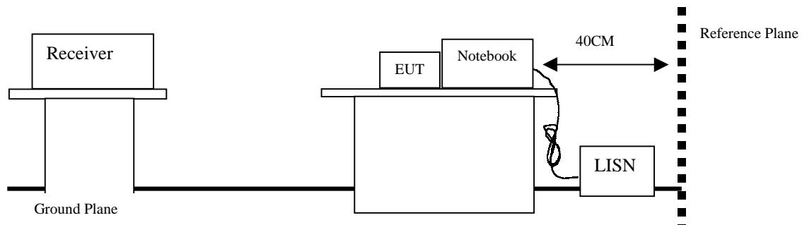
The EUT are connected to the main power through a line impedance stabilization network (LISN). This provides a 50 ohm/50uH coupling impedance for the measuring equipment. The peripheral devices are also connected to the main power through a LISN that provides a 50ohm/50uH coupling impedance with 50ohm termination.
