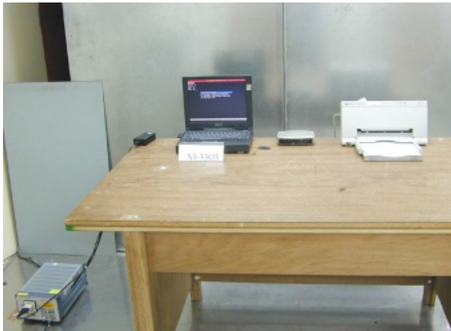
Photo 1: Conducted Test Set-up (front)
