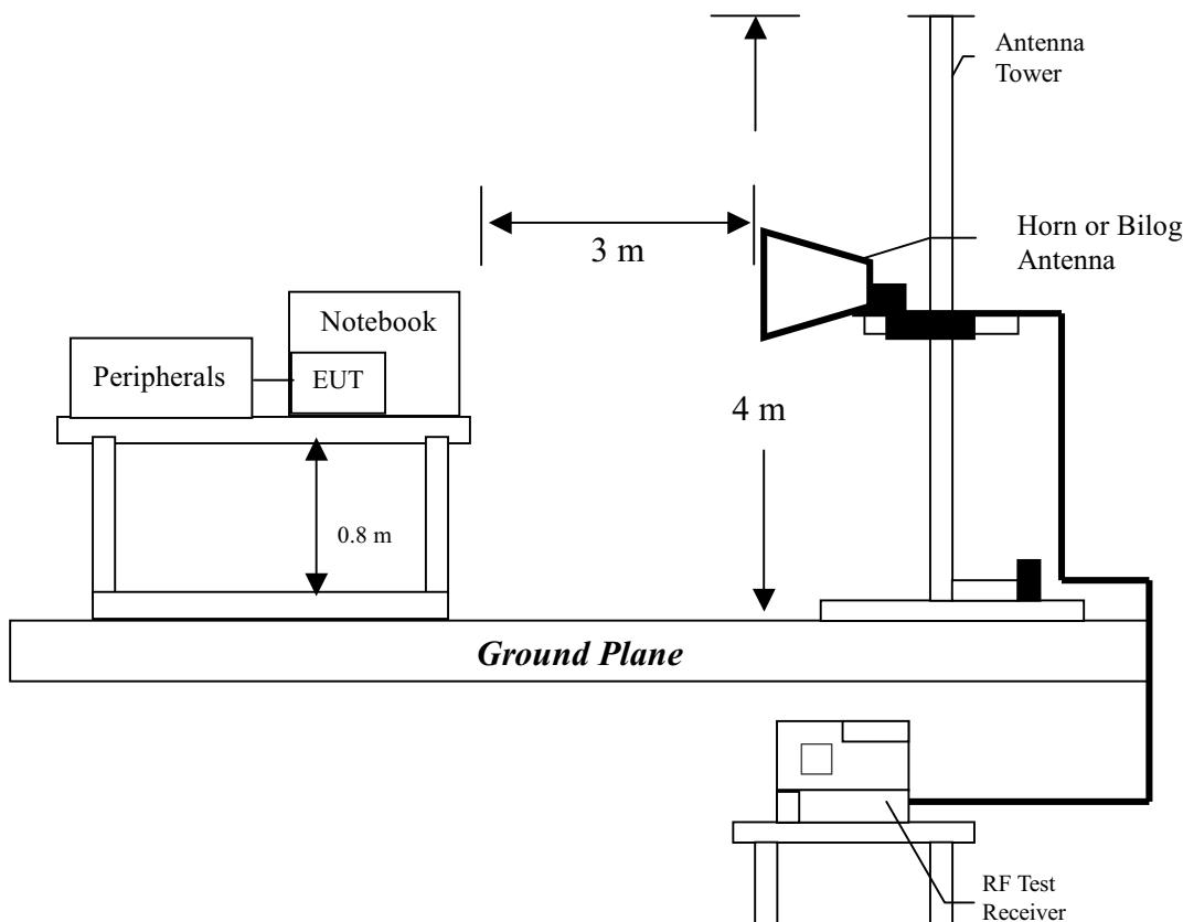
The signal is maximized through rotation and placement in the three orthogonal axes. The EUT and its peripherals are placed on a turn table which is 0.8 meter above ground. The turn table can rotate 360 degrees to determine the position of the maximum emission level. The EUT was positioned such that the distance from antenna to the EUT was 3 meters. The antenna can move up and down between 1 meter and 4 meters to find out the maximum emission level.
