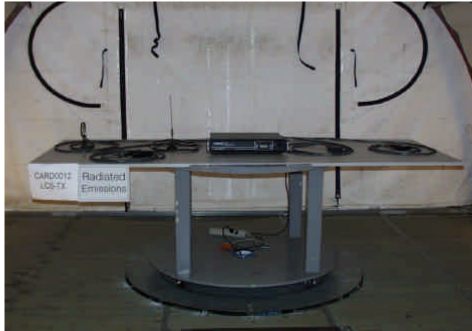
Radiated Emissions, Test Setup.
