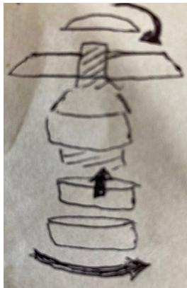
Insert the WVL threaded column up through the hole. Screw on the antenna cap above the valve box lid.
