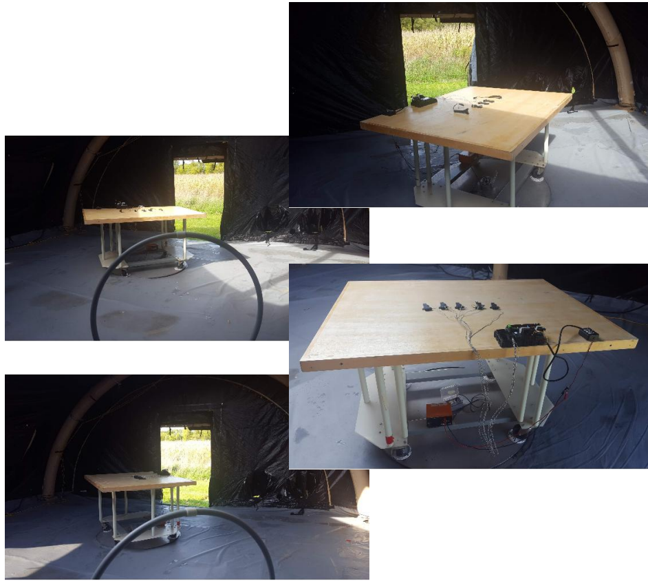
Figure 4: Radiated Emissions Test Setup Photograph(s).
