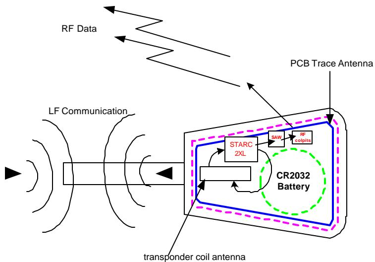
**Figure 2. SKREEK Block Diagram****SKREEM Variants:**
