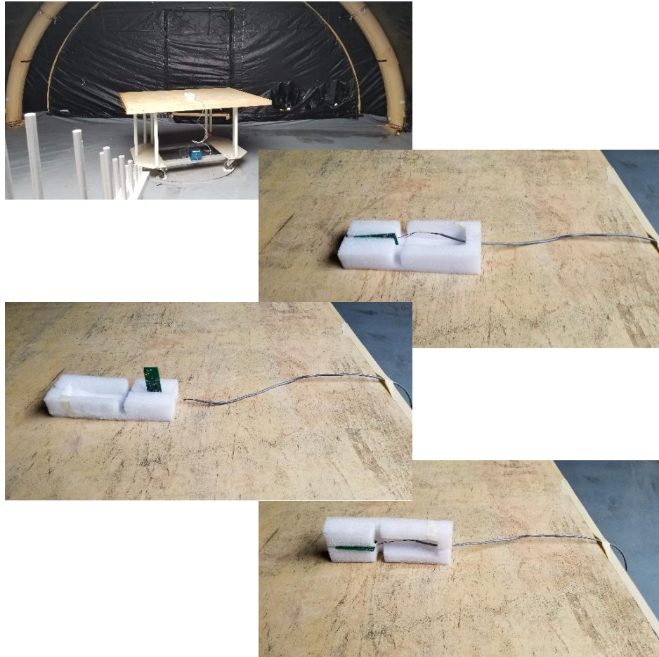
Figure 4: Radiated Emissions Test Setup Photograph(s).
