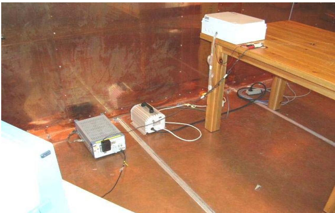
**Model: S1566 - Radiated spurious emission 30-1000 MHz**
