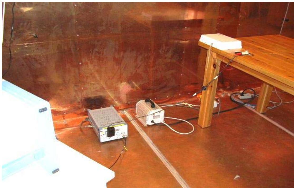
**Model: S1513 - Radiated spurious emission 30-1000 MHz**
