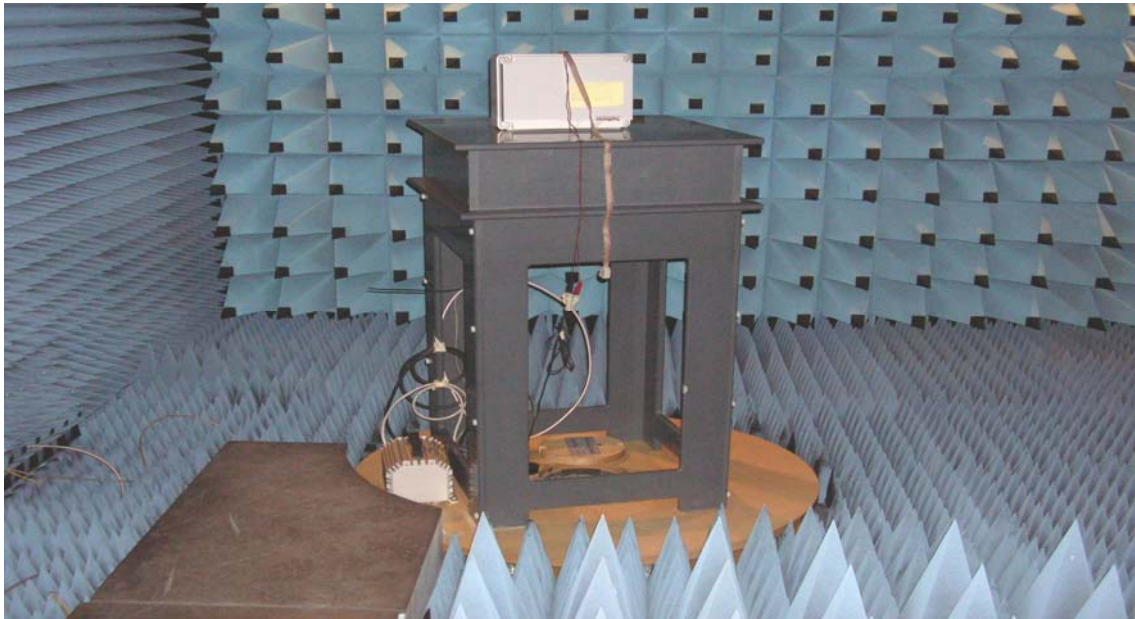
Model: S1513 - Radiated spurious emission 1-26 GHz
