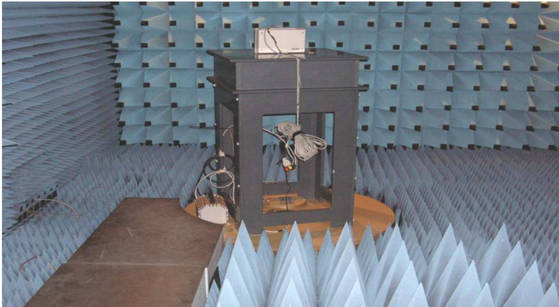
Model: S1500 - Radiated spurious emission 1-26 GHz
