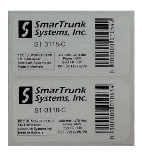
FCC ID: M38-ST-3118C FM Transceiver Smartrunk Systems Inc. Made In Malaysia
