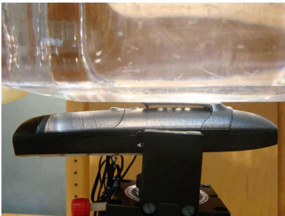
Body-worn Setup Photo (Model: CL-65P)
