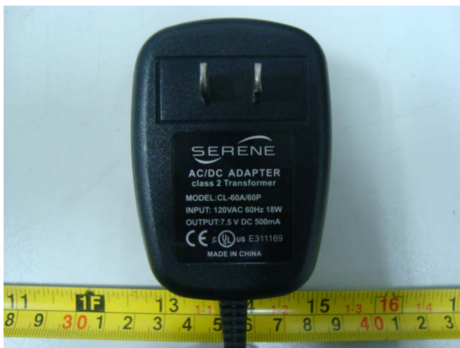
EUT – AC/DC Adapter View
