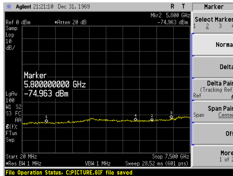
Figure 5-9 Harmonic Emissions at Antenna Terminals
