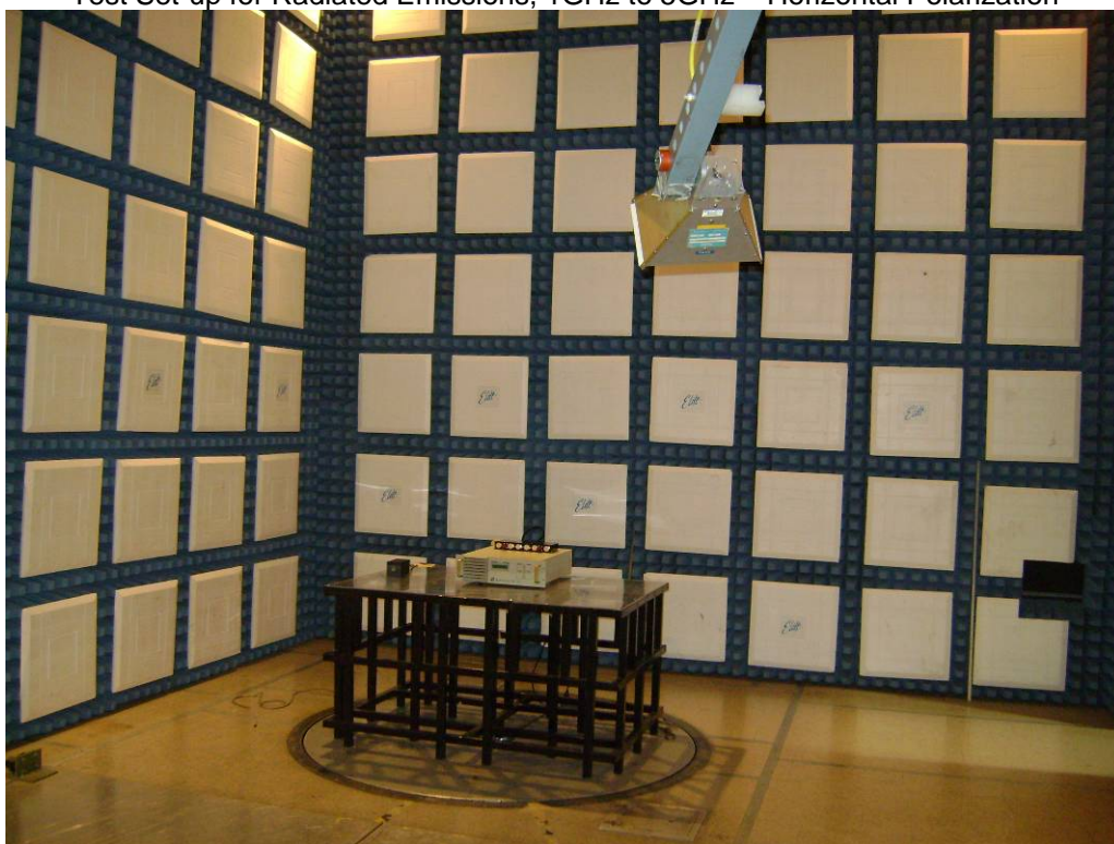
Test Set-up for Radiated Emissions, 30MHz to 5GHz – Vertical Polarization
