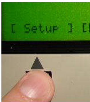
Fig.6.8: Hit the SETUP soft-key to start the ALC-OFF operation
