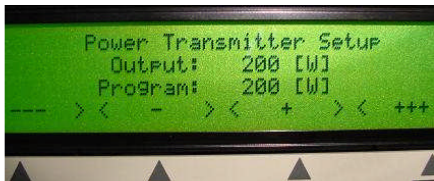
Fig.6.6: Power Setup Screen at the end, it must coincide with the external wattmeter reading
