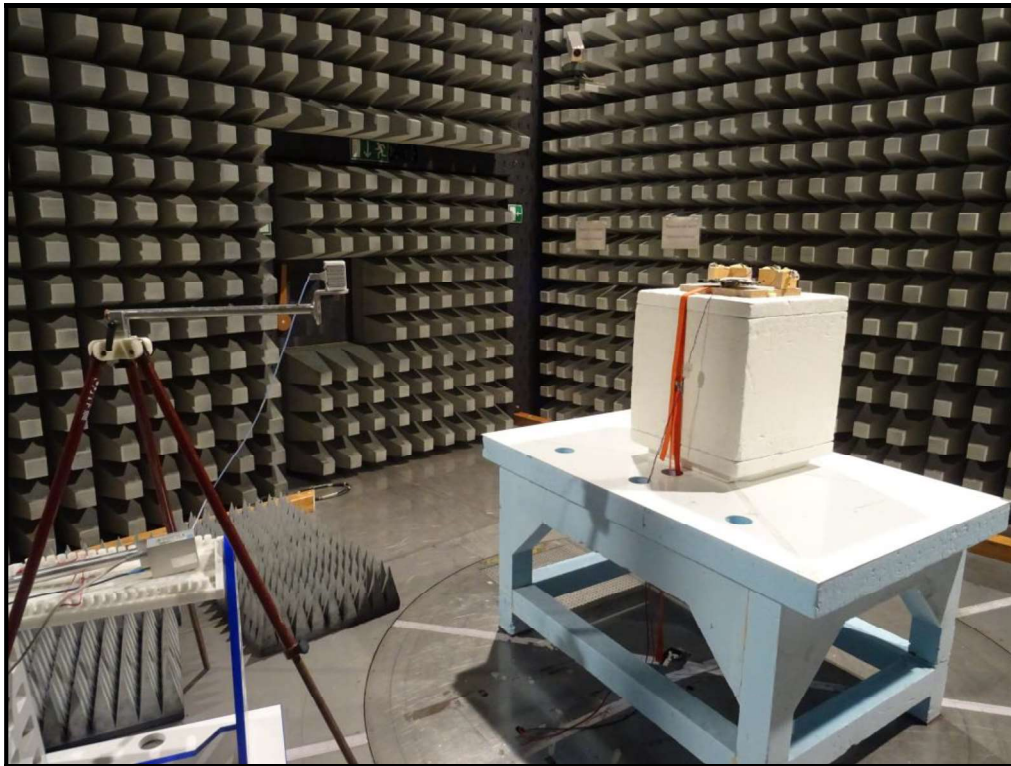
Photo 8: Terminated Ports 1+2+3+4 with 50 \Omega
