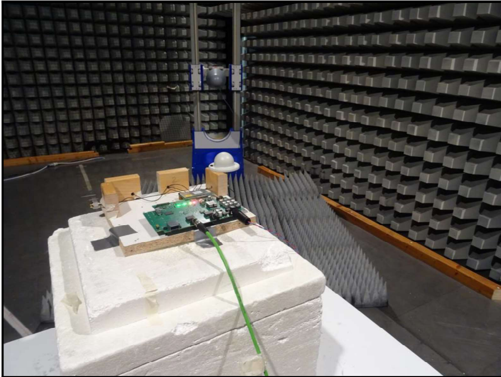
Photo 13:EUT- SISO PORT 1 (Ports 2,3 & 4 Terminatd with 50 \Omega )
