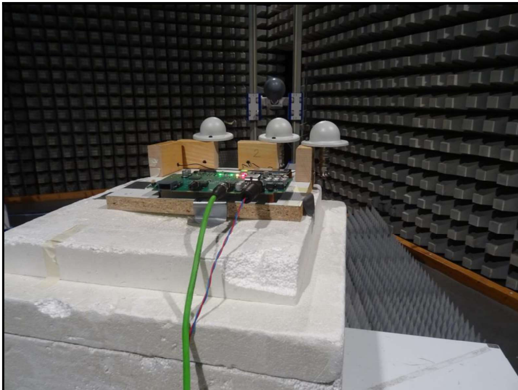
Photo 21:EUT- MIMO PORT 1+2+3 (Port 4 Terminatd with 50 \Omega )
