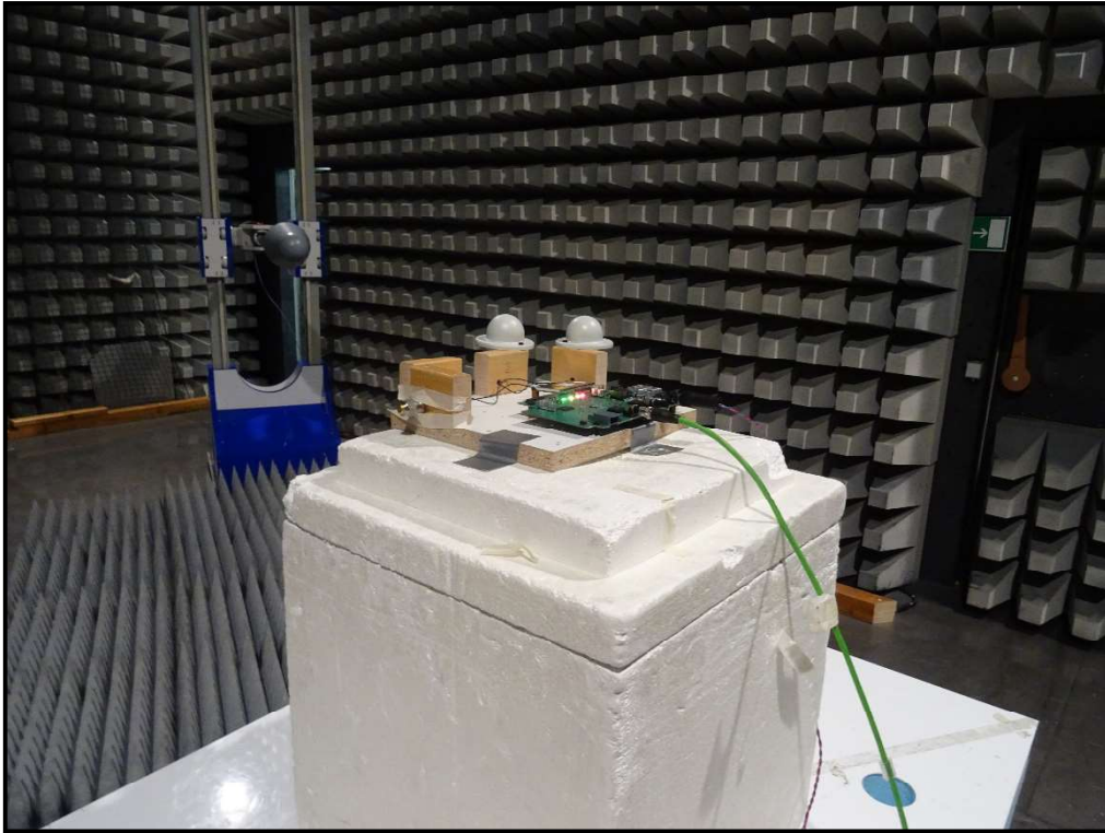
Photo 17: EUT- MIMO PORT 1+2 (Ports 3 & 4 Terminated with 50 \Omega )
