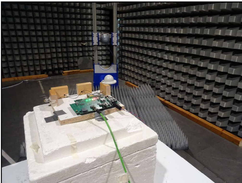
Photo 13: EUT- SISO PORT 1 (Ports 2,3 & 4 Terminated with 50 \Omega )
