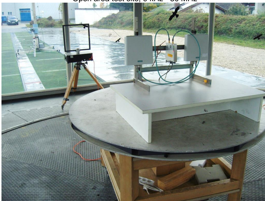
Open area test site, 30 MHz - 1000 MHz
