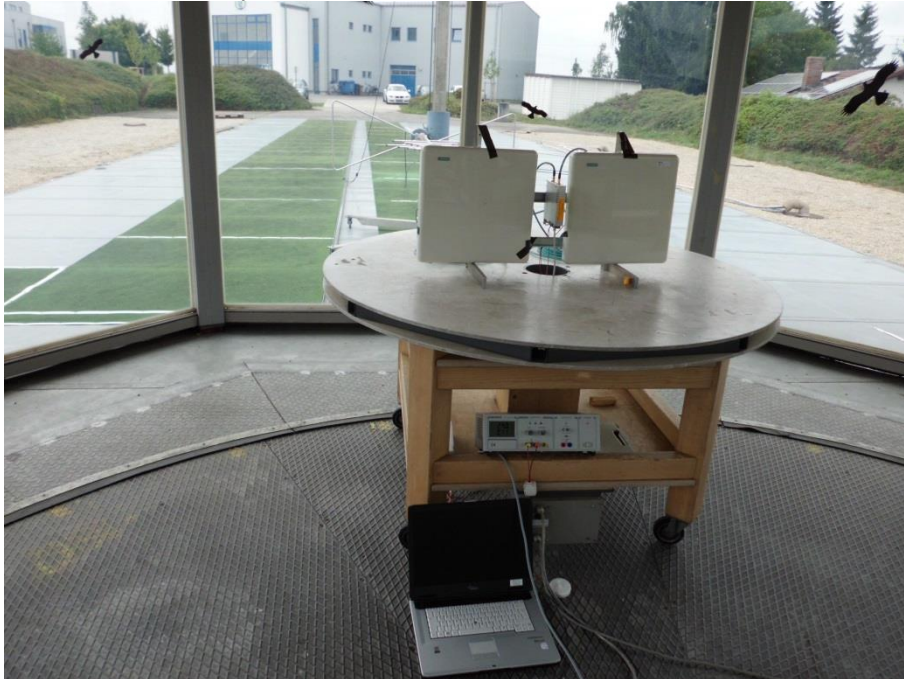
Open area test site, 30 MHz - 1000 MHz
