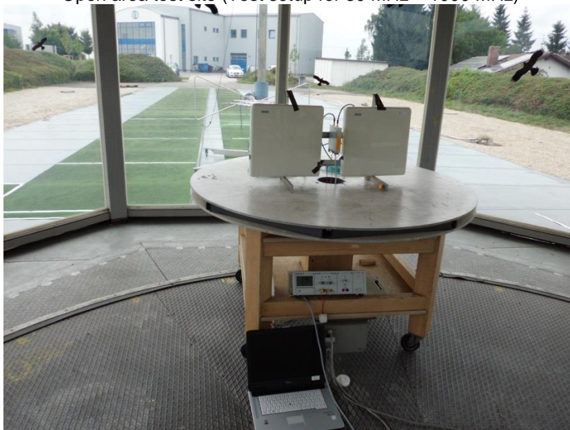
Open area test site (Test setup for 30 MHz – 1000 MHz)
