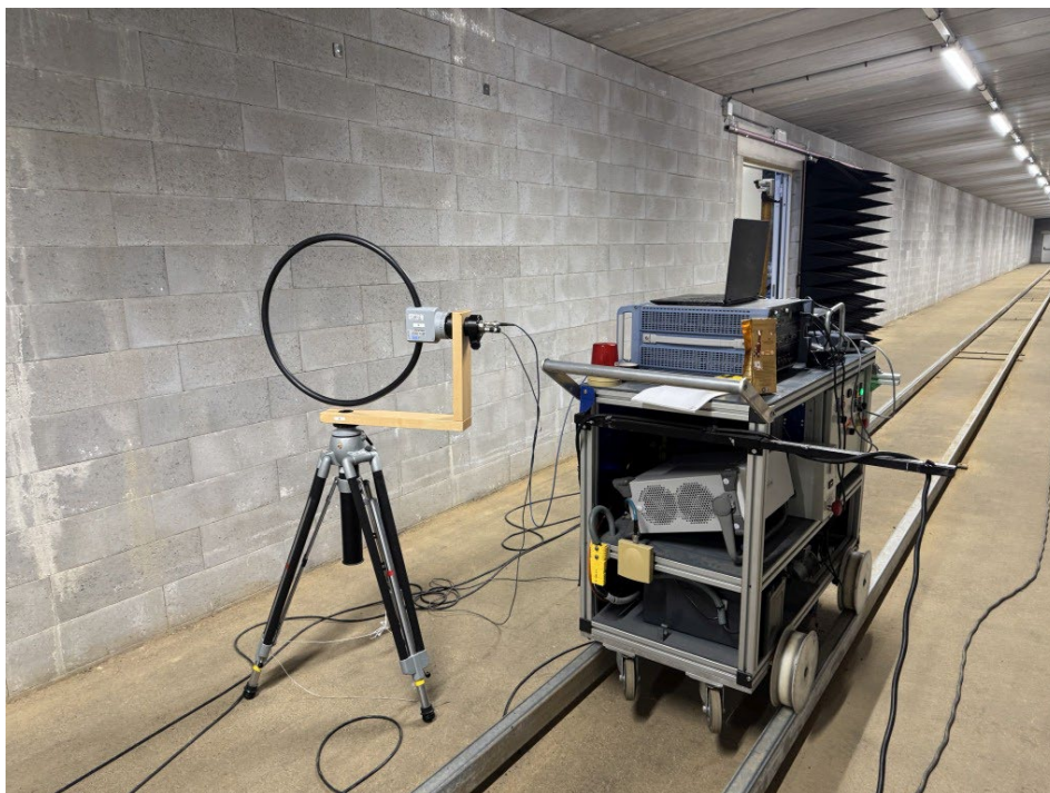
Photo 7: HFH2-Z2 magnetic field antenna 9.0 kHz – 30 MHz
