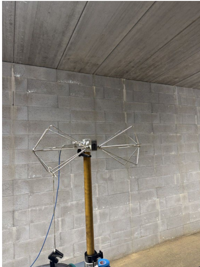
Photo 6: VUBA 9117 biconical dipole antenna 30.0 MHz – 1.0 GHz on trolley
