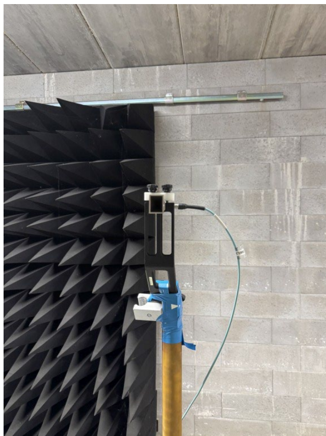
Photo 6: Standard gain horn 26.5 GHz – 40.0 GHz on trolley
