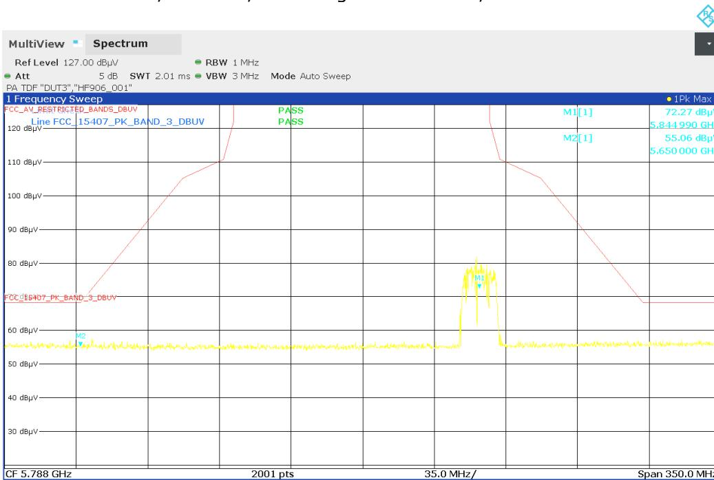
Radio Technology = WLAN a, Operating Frequency = low, Subband = U-NII-1
