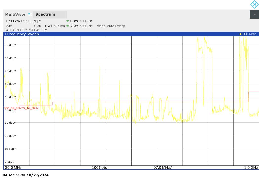
Radio Technology = WLAN a, Operating Frequency = mid, Subband = U-NII-1,
