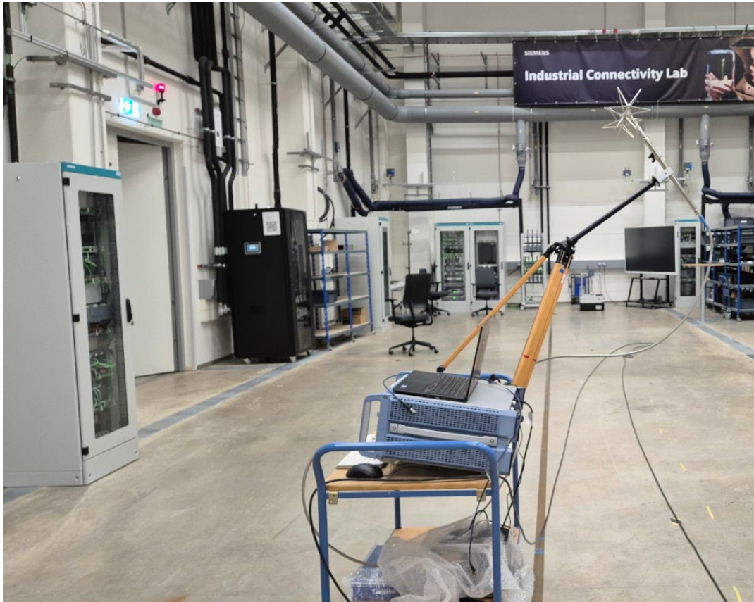
Photo 6: VUBA 9117 biconical dipole antenna 30.0 MHz – 1.0 GHz on trolley
