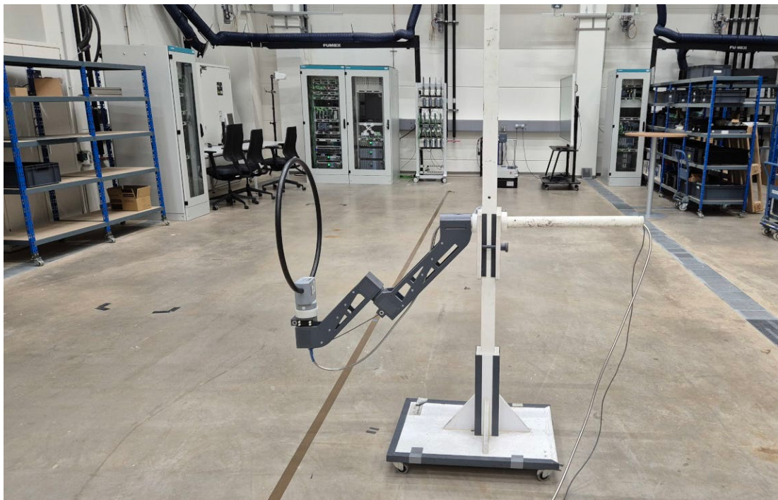
Photo 7: HFH2-Z2 magnetic field antenna 9.0 kHz – 30 MHz
