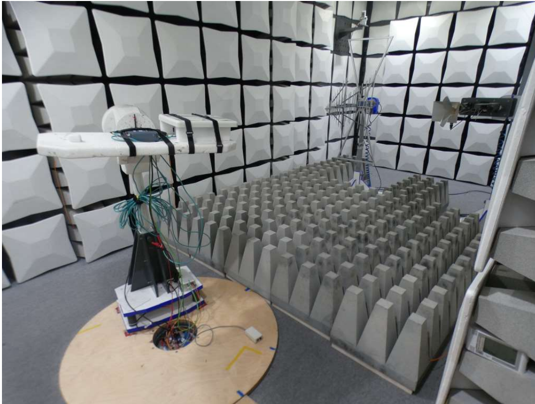
Photo 10: Test setup for radiated emissions measurements in fully anechoic chamber (1 GHz to 26 GHz), right side view, [Setup S02_AJ01]
