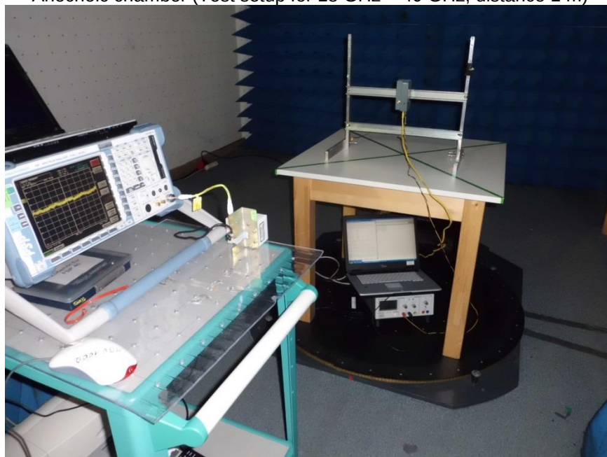
Anechoic chamber (Test setup for 18 GHz – 40 GHz, distance 1 m)
